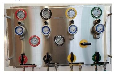
The H2V controller incorporates metal gas flow tubes designed for high pressures and hazardous applications and provides a significant safety factor to explore flow and pressure ranges outside the traditional range of most current controllers.
