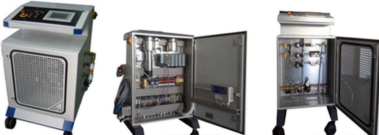
Spraywerx ID-Nova Compact Controller is a mass flow controlled computerized HVOF spray system capable of operating HVOF guns such as ID-Nova, Mini-Nova and DJ. The ergonomically styled operator panel contains the complete electrical, oxygen, fuel, cooling and carrier gas control. The main components of the electrical control are the Siemens Operator Panel KTP 700 Basic DP and the Siemens PLC type S7.
