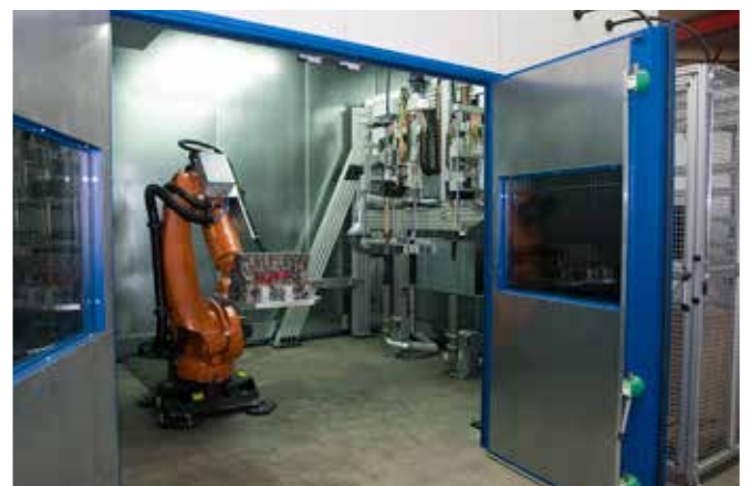
RSW Turn Key Coating Center for engine remanufacturing
